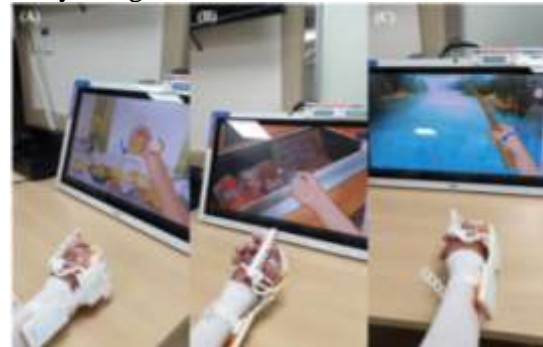
Gambar 1. Volitional movements in the virtual reality-based rehabilitation system: (A) finger flexion/extension, (B) forearm pronation/supination, (C) wrist flexion/extension (Joo et al., 2020)
